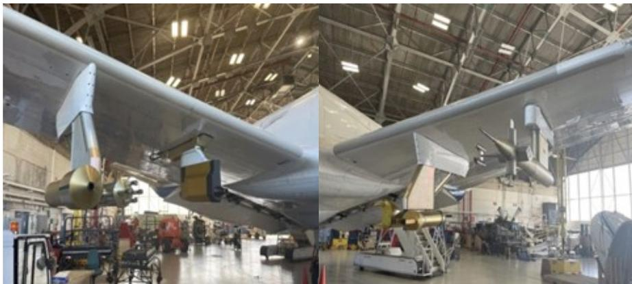
The left and right wings of the P-3 aircraft capture data in different ways, some particles entering directly into their openings, some read by lasers, and more. Photo Credit: Christian Nairy.
