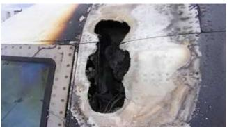
A pilot sent these photos of an Atlantic Southeast Airlines/Delta Connection aircraft, after it suffered a lightning strike.
